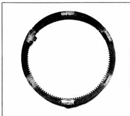
Ring gear (above), spur gears (below) require special attention during an overhaul. Reduction gear set which lies between the motor and the spur gears.
